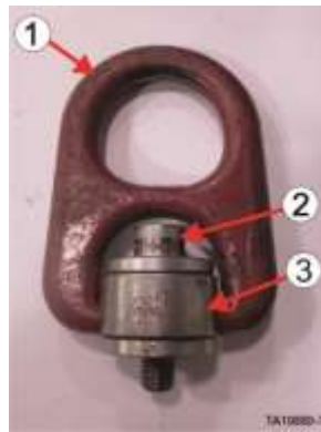
1) Swivel mount, 2) Lifting clevis, 3) Capscrew (allen head 1"-14 NS – 2B GR8)
