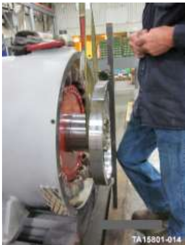
Figure 244. Measurement between a straight edge and generator stator
