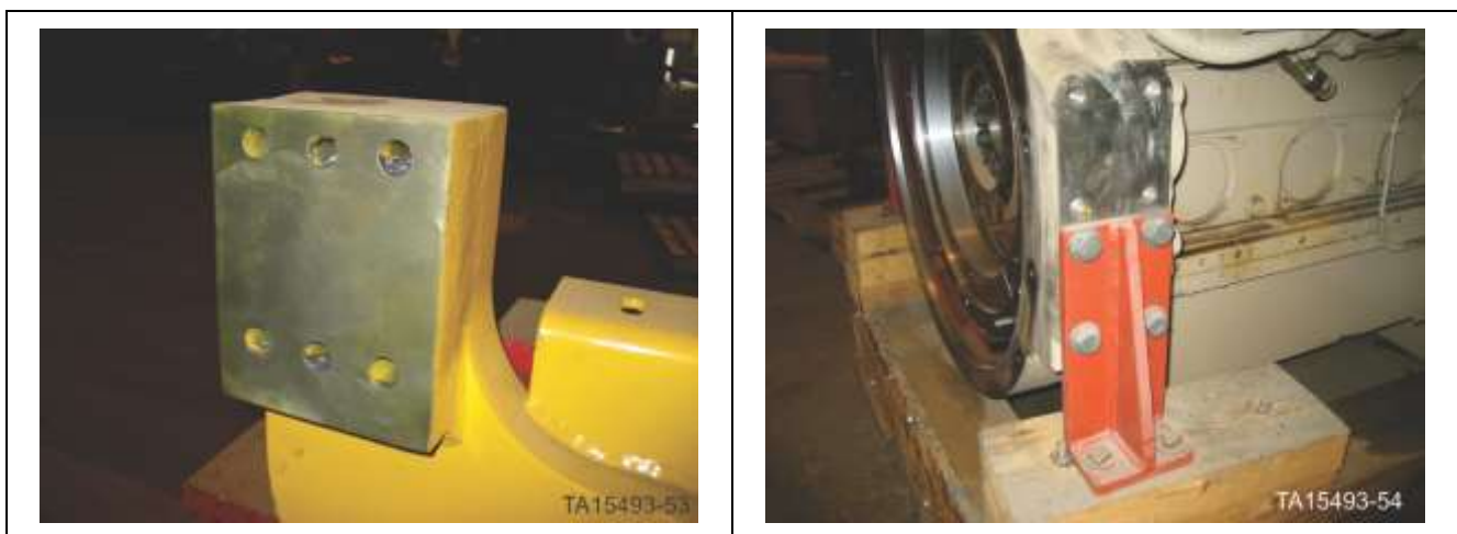
Figure 254. Clean Mounting Faces on the Engine Mounts and the Flywheel Housing
