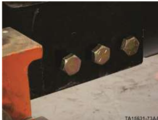
Figure 298. Final torque - engine mount bolts
