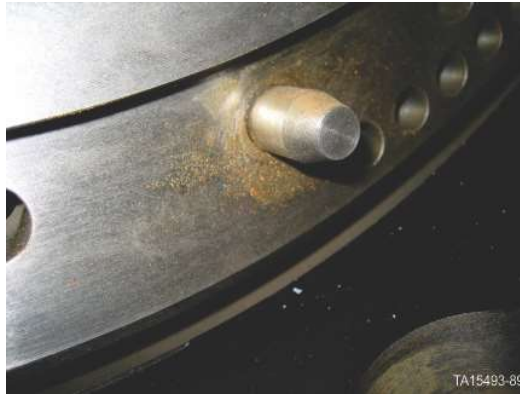
Figure 291. Alignment studs are built into the flex plate
