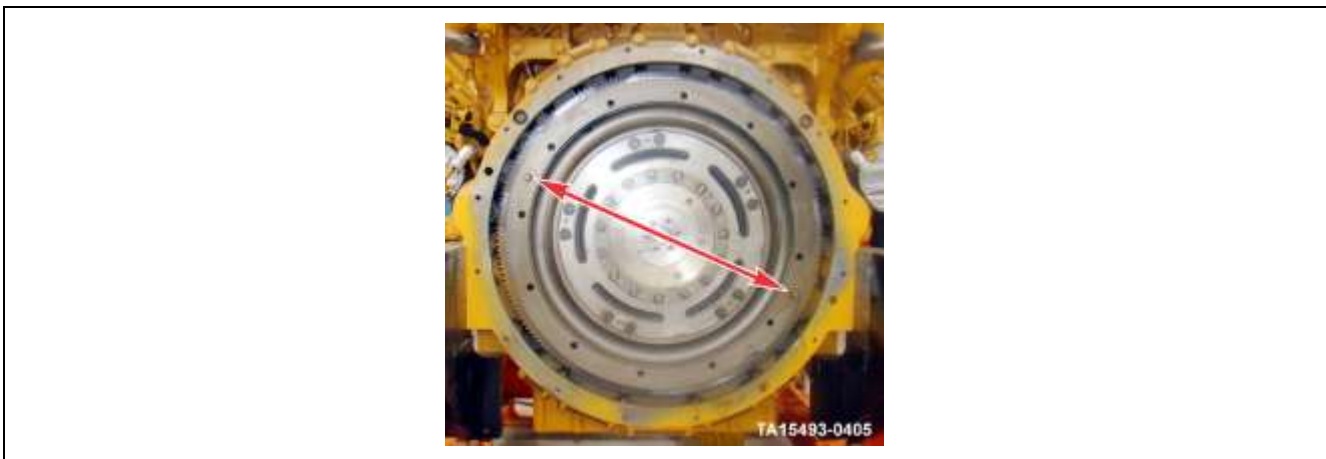
Figure 278. Dowel Pin Location in Flexplate - Typical
