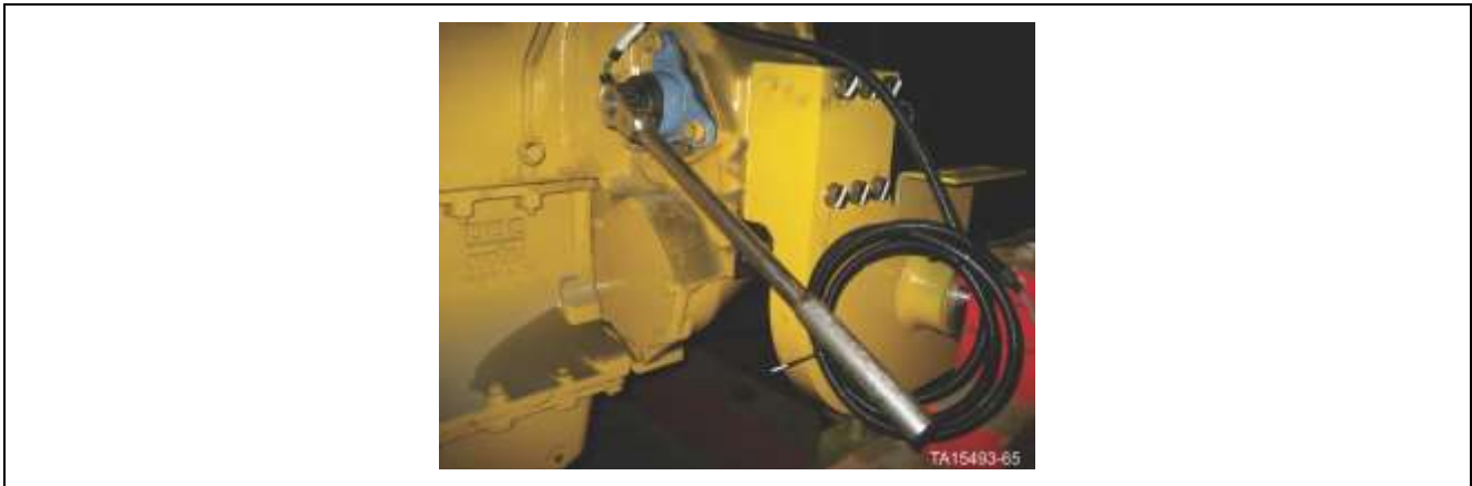
Figure 264. Rotating Engine Crankshaft with Manual Drive Gear
