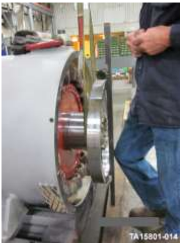
Figure 133. Measurement between a straight edge and generator stator
