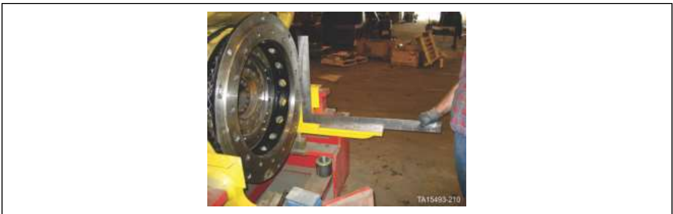
Figure 170. Check perpendicular alignment of mount feet and stator adapter - (2 of 2)
