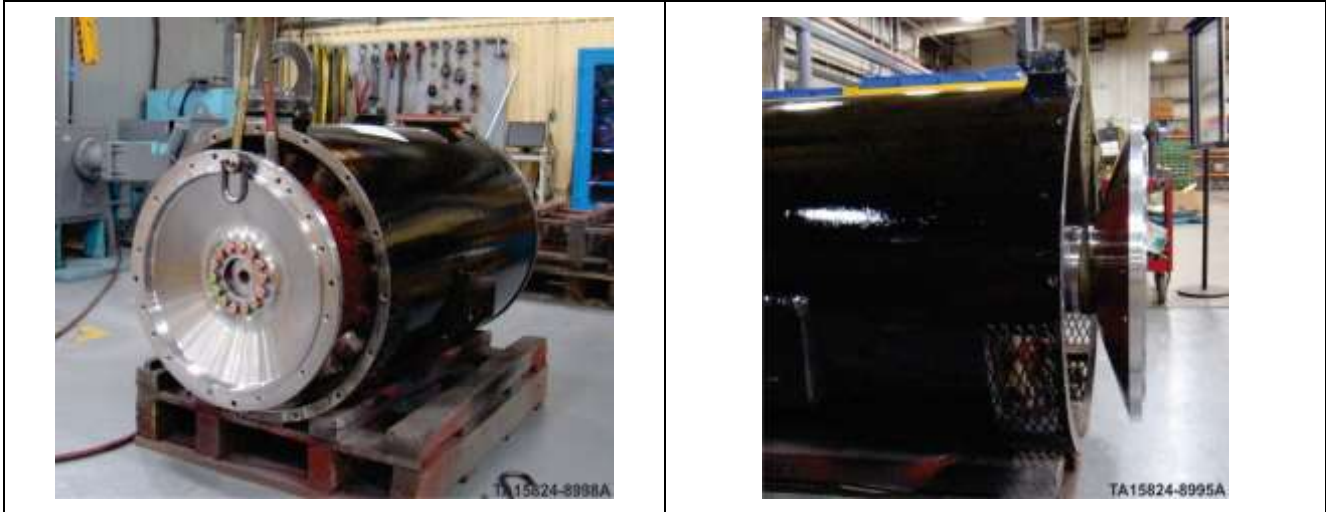
Figure 235. Lifting strap located on drive end
