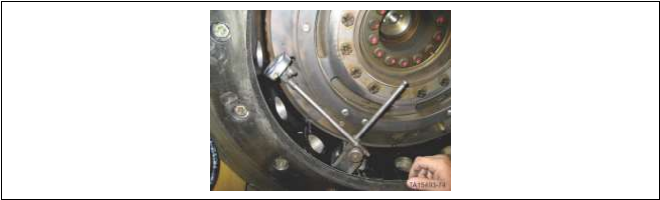
Figure 161. Measurement of axial runout of engine flexplate mating surface
