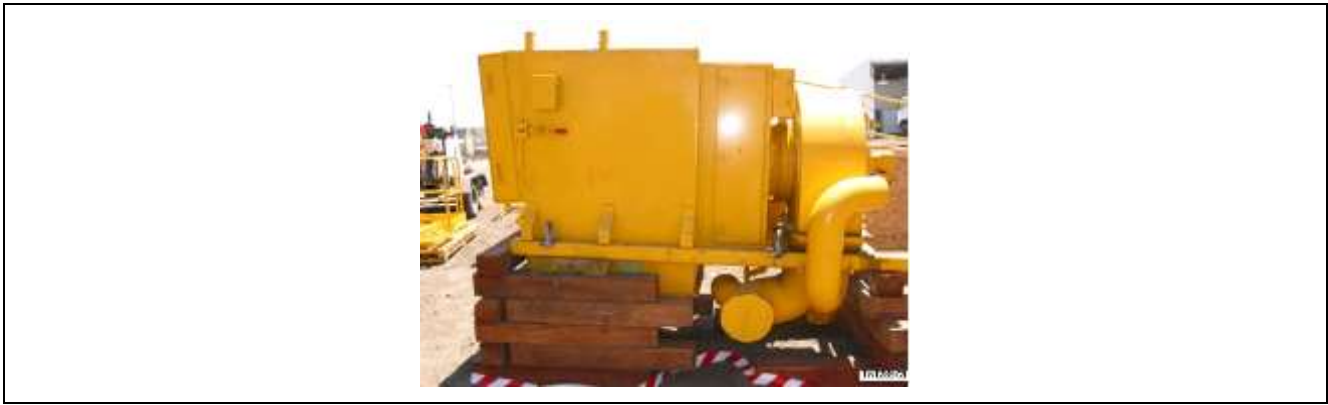
Figure 63. KLENZ™ and blower assembly supported by cribbing - 1 of 3
