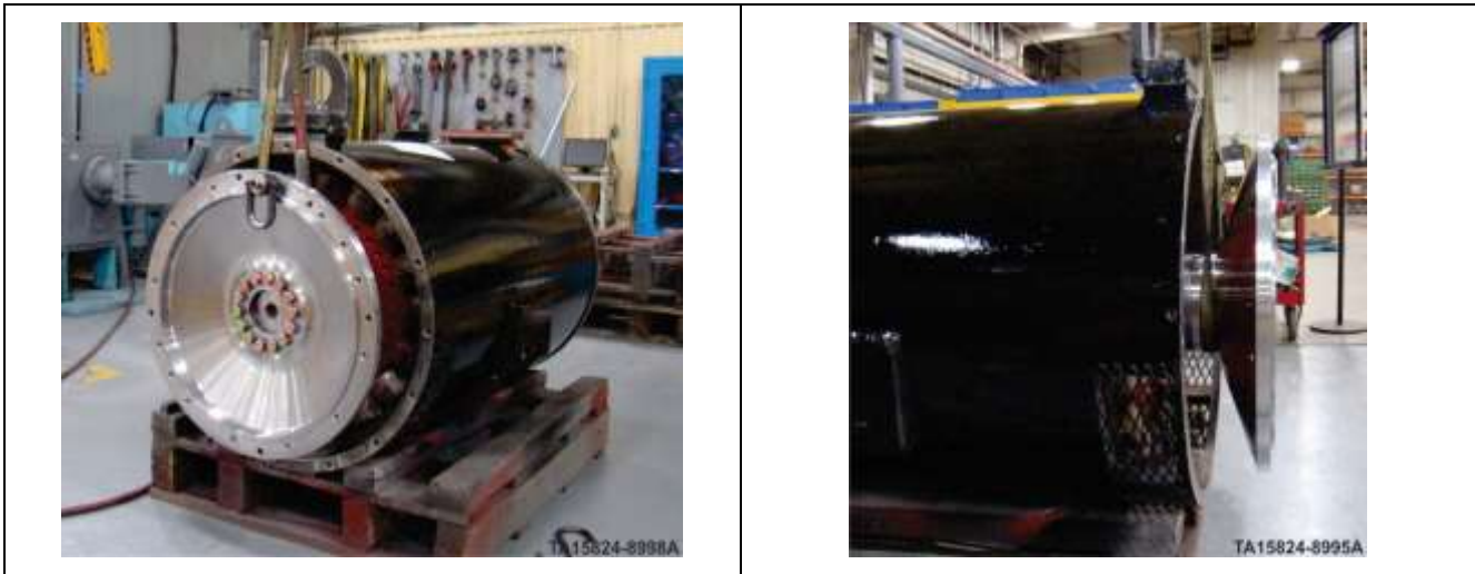
Figure 90. Nylon strap around the rotor shaft (typical)
