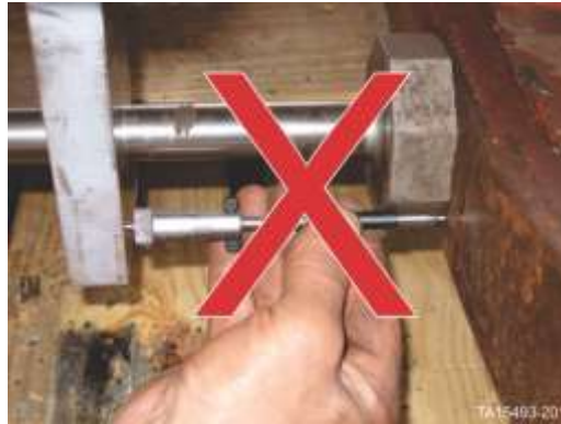
Figure 132. Do not measure between endplay brace as it is most likely not a straight edge
