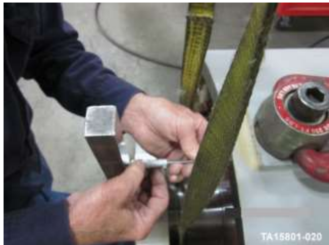
Figure 133. Measurement between a straight edge and generator stator
