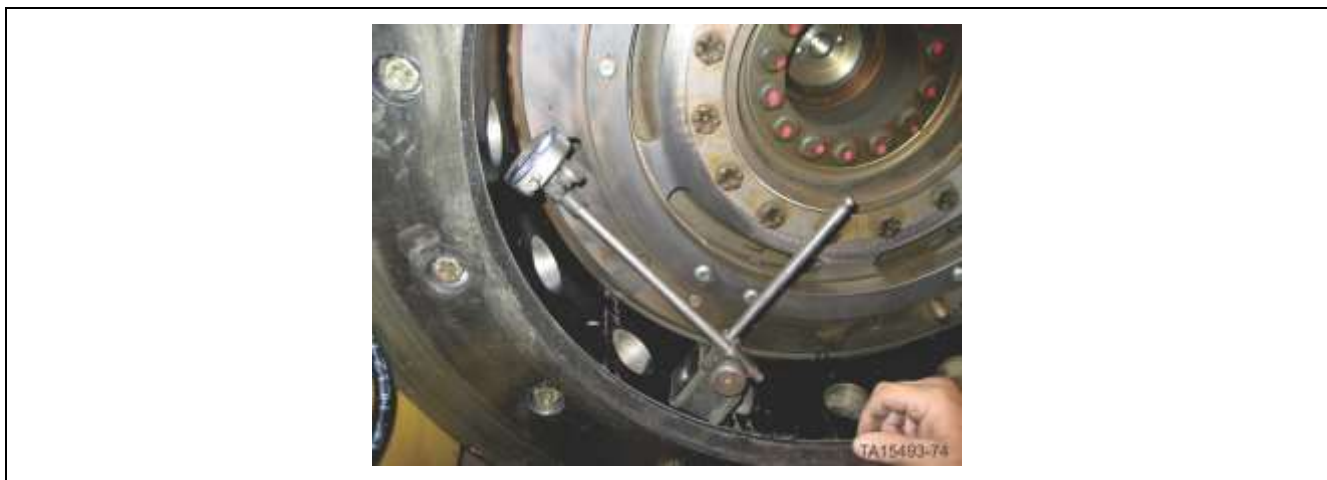
Figure 269. Measurement of Axial Runout of Engine Flexplate Mating Surface
