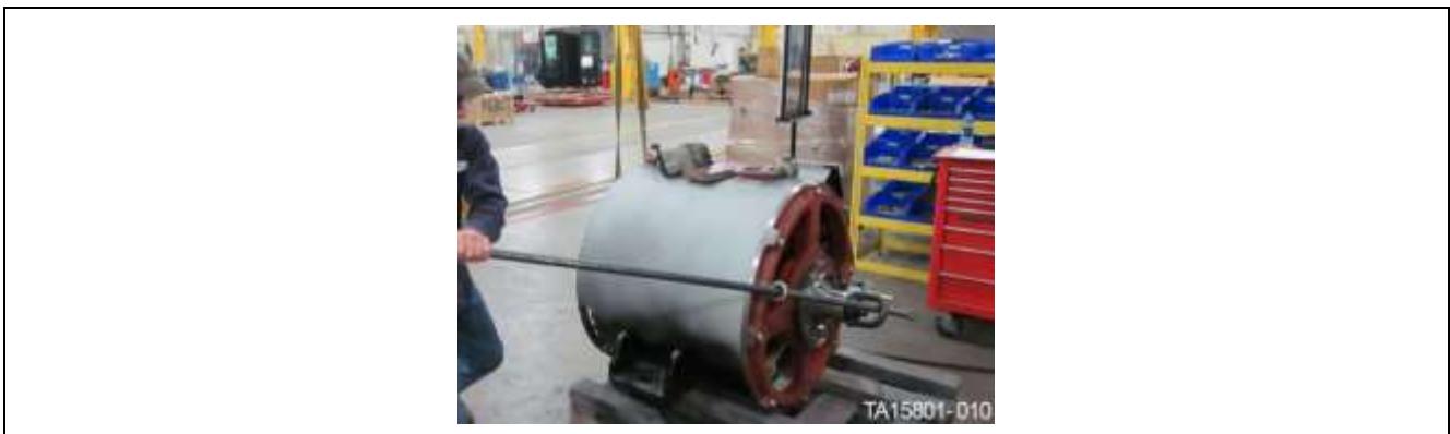
Figure 131. Shift rotor toward non drive end
