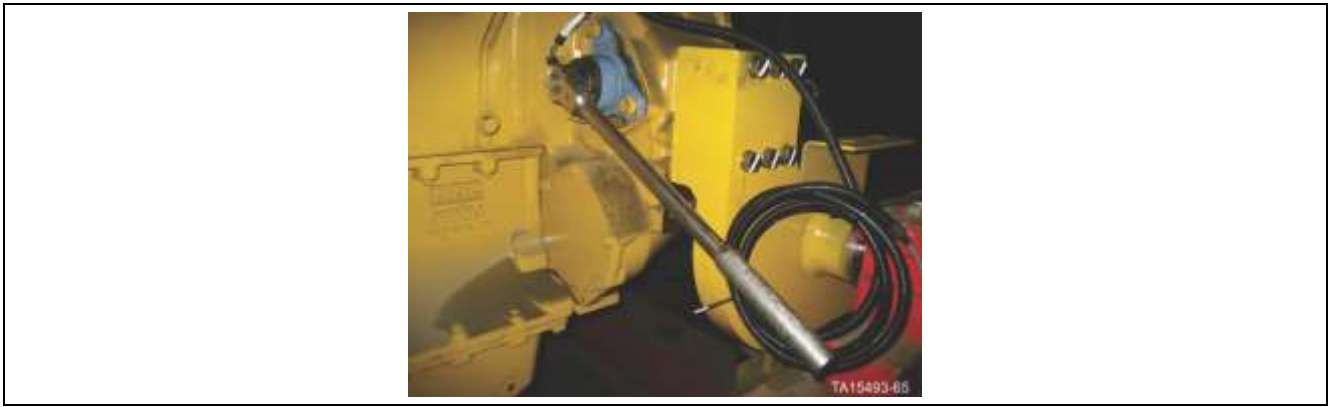
Figure 40. Rotating engine crankshaft with manual drive gear
