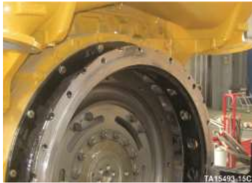
Stator adapter plate is bolted to engine
