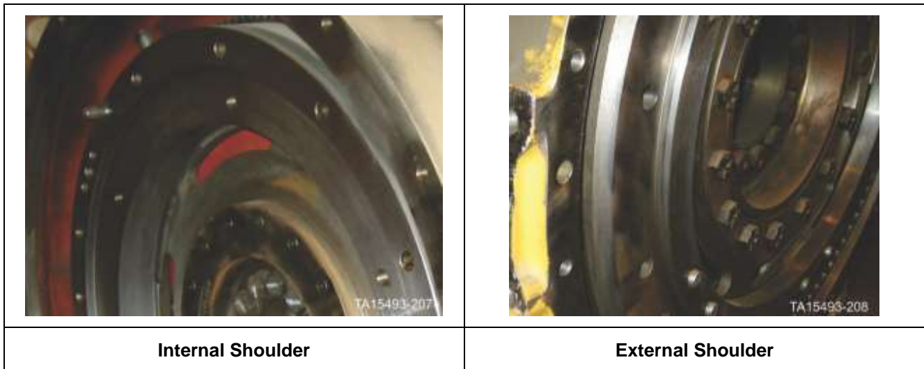
Figure 268. Measurement of Axial Runout of Engine Flexplate Mating Surface
