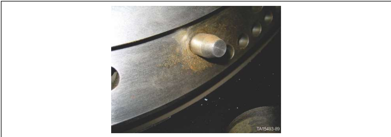
Figure 185. Alignment studs are built into the flexplate
