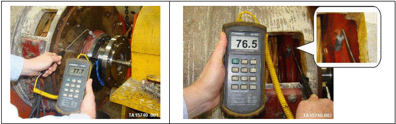
Figure 309. Typical temperature bearing testing
