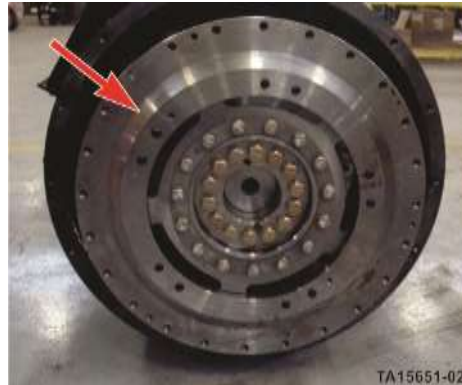
Flex Plate is Part of Rotor Adapter
