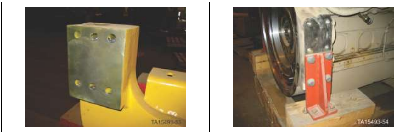
Figure 146. Clean mounting faces on the engine mounts and flywheel housing
