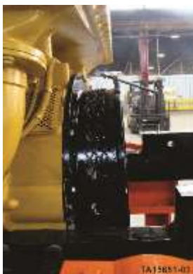
Side view - stator adapter plate bolted to engine
