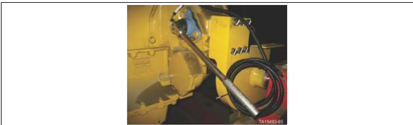
Figure 82. Rotating engine crankshaft with manual drive gear
