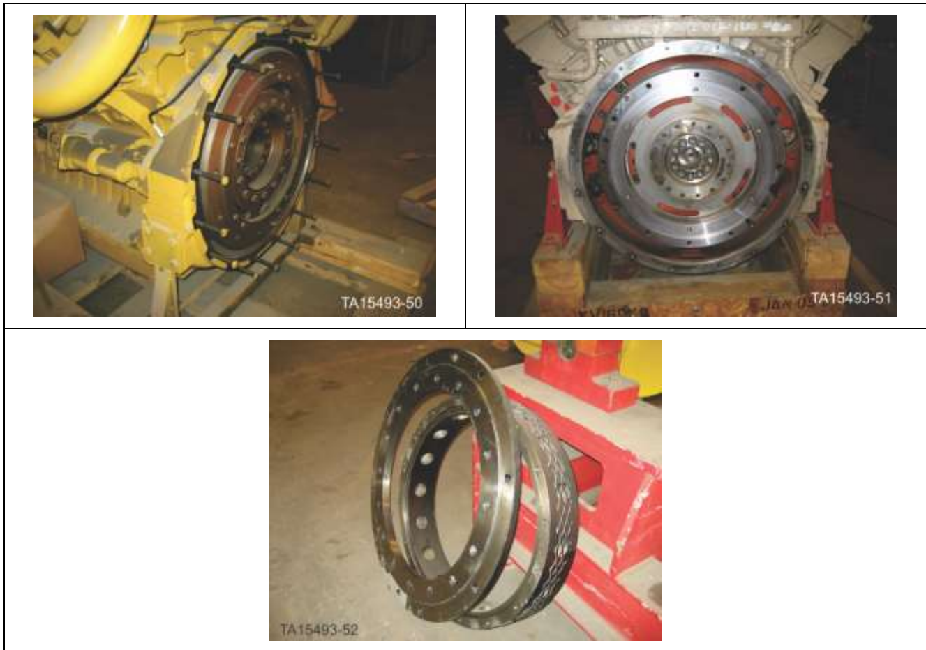
Figure 253. Clean All Mounting Faces and Shoulders
