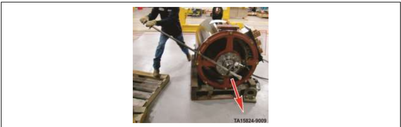
Figure 242. Shift rotor toward non drive end
