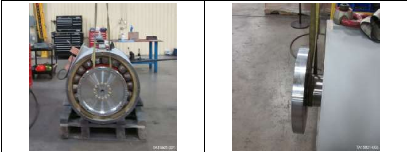
Figure 124. Lifting strap located on Drive End
