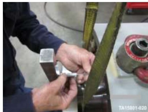
Figure 244. Measurement between a straight edge and generator stator
