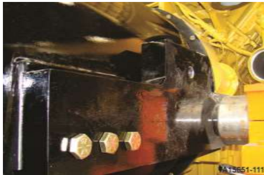
Figure 304. Final torque - engine mount bolts
