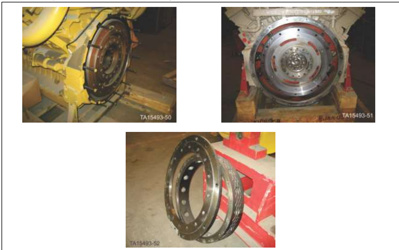
Figure 145. Clean all mounting faces and shoulders
