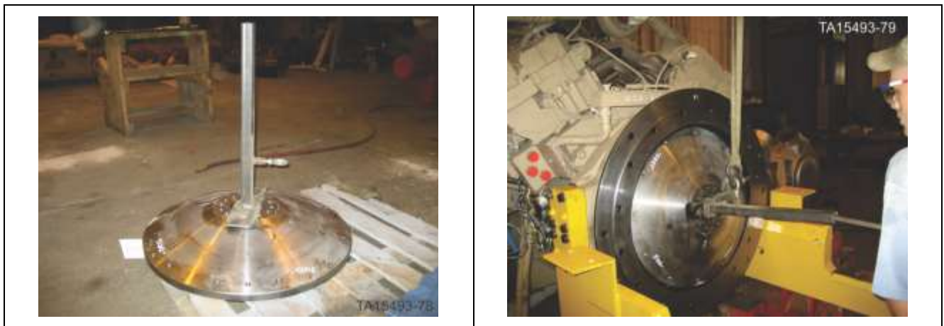
Figure 280. Lift and install rotor adapter
