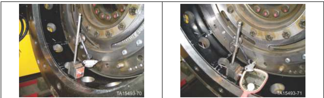
Figure 158. Measurement of radial runout of engine flexplate
