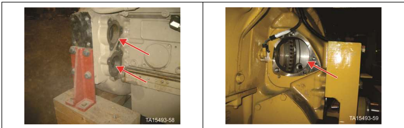
Figure 260. Remove Cover/Starter to Access Back Side of Flexplate
