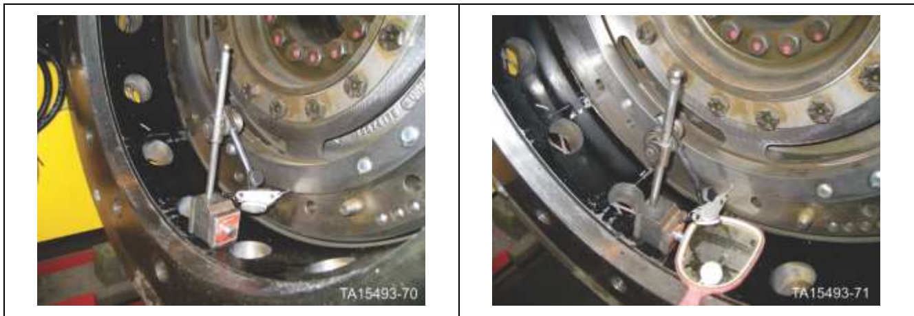
Figure 266. Measurement of Radial Runout of Engine Flexplate
