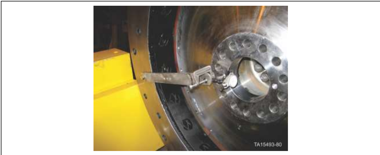
Figure 177. Checking I.D. runout of rotor adapter plate
