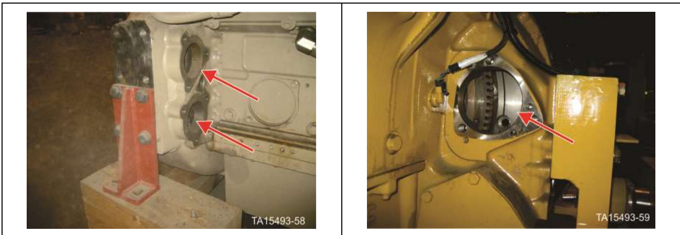
Figure 152. Remove cover/starter to access back side of flexplate
