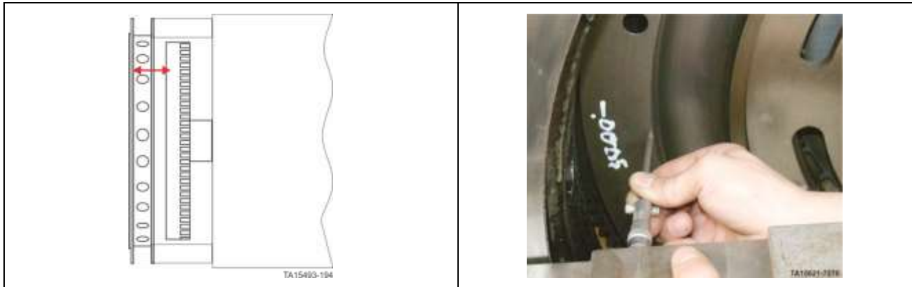
Figure 288. Measure distance between stator adapter and flexplate
