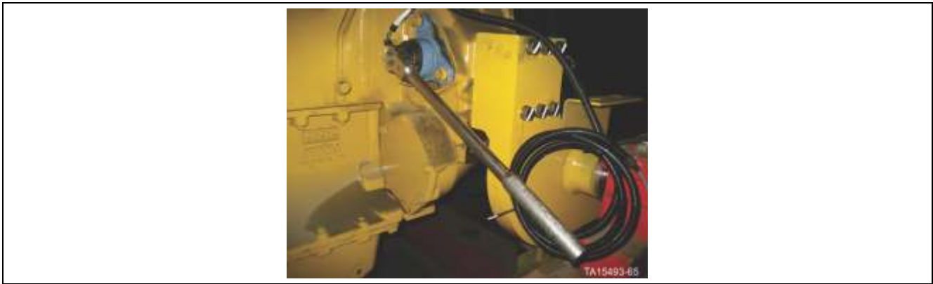
Figure 156. Rotating engine crankshaft with manual drive gear
