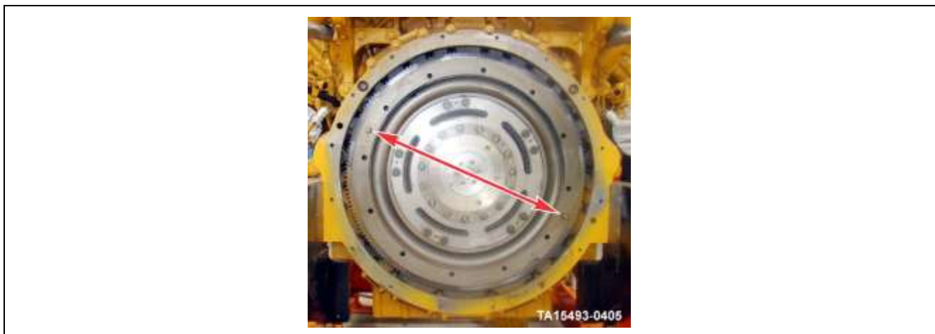
Figure 174. Dowel Pin Locations in Flexplate - Typical
