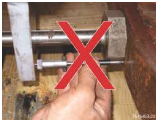
Figure 243. Do not measure between endplay brace as it is most likely not a straight edge
