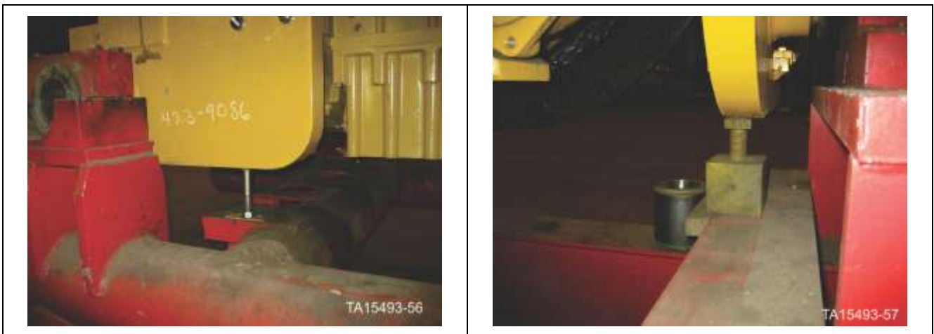
Figure 256. Jack Bolt Directly Under Engine Mount
