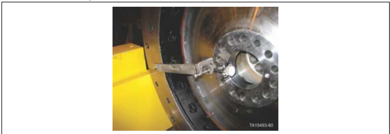
Figure 281. Checking I.D. runout of rotor adapter plate - (1 of 2)
