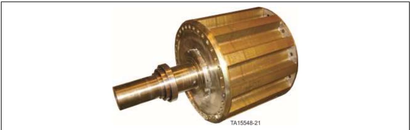
Figure 4. SR generator laminations
